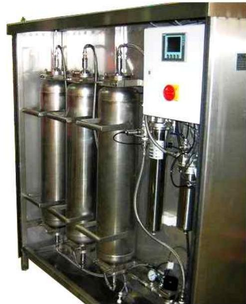
*ATMoS with options humidity-/temperature-sensor, bigger particle filter, industrial SPS with touchpanel and leakage monitoring (weatherproof housing, drip tray and leakage sensor)*
